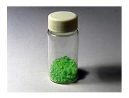
**Purpose:** To prepare the complex trisoxalatoferrate(III),  $Fe(C_2O_4)_3^{-3}$  anion and isolate it as its hydrated potassium salt,  $K_3[Fe(C_2O_4)_3].3H_2O$ . Also, to study the photochemical reduction of the sample.
